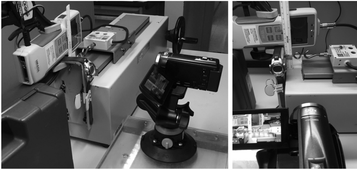
Fig. 2. Load cell with digital force gauge, stopwatch, scale bar, hand wheel test stand, and video camera.
