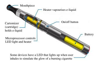
**Fig. 1.** Structure of an electronic cigarette (EC). ECs are made of a plastic tube, an electronic heating element, a liquid cartridge, and a battery. The rechargeable lithium battery (with or without an LED indicator) powers the heating element that heats and vapourizes the liquid in the cartridge to produce an aerosol that the user then inhales. The liquid contains solvents and optional nicotine and flavouring agents. Modified from Federal Emergency Management Agency (2014).
