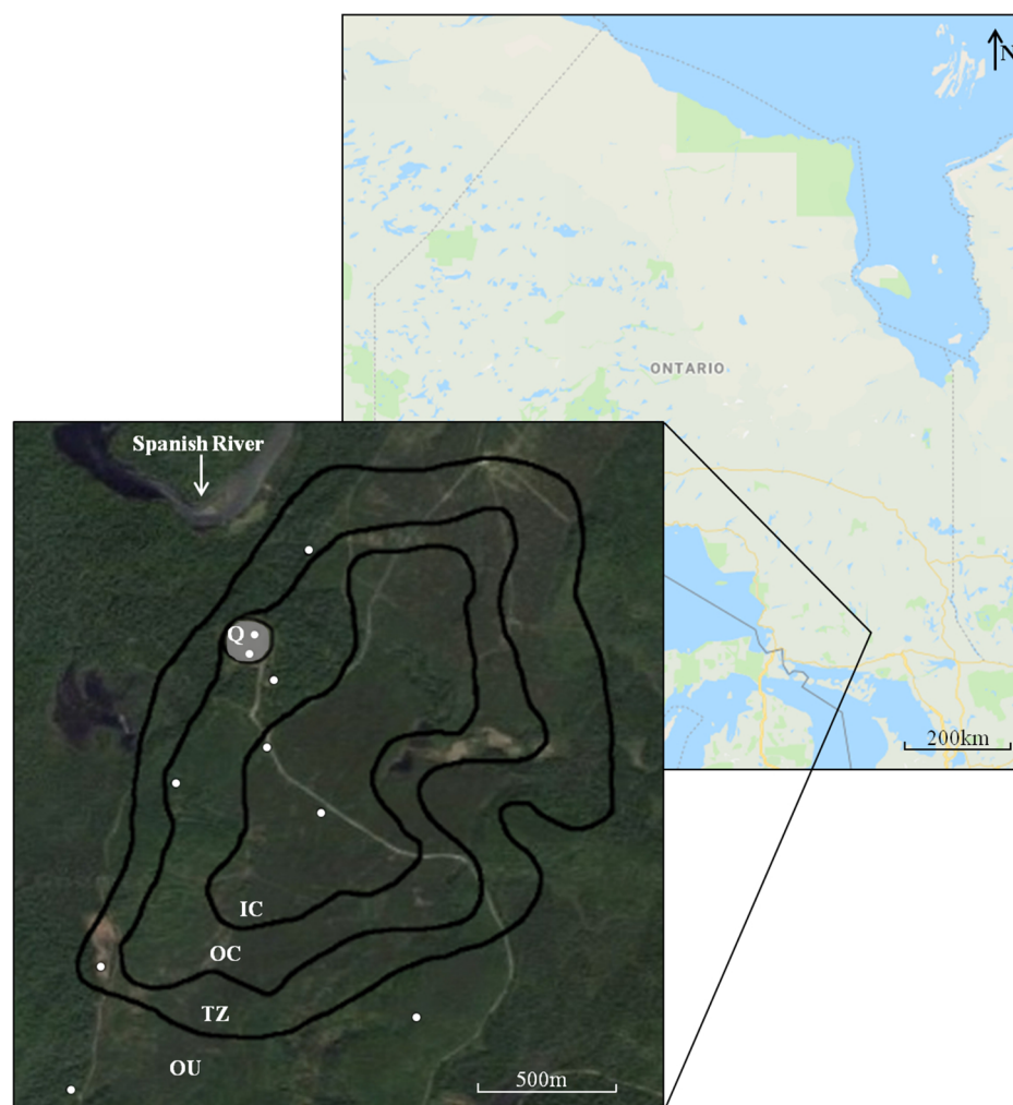
Fig. 1. Overview of the Spanish River Carbonatite (SRC) deposit located near the Spanish River in Ontario, Canada. Five zones were considered for the study and are delineated by the black lines: the quarry (grey circle) where SRC is actively mined (Q), the inner core (IC), the outer core (OC), the transition zone (TZ), and the outside of the deposit (OU). Sampling sites are indicated by the white dots. Zones estimated from data provided by Agricultural Mineral Prospectors Inc. (2004) . Map data provided by Google (2018) and satellite data provided by DigitalGlobe and CNES/Airbus (2018).
