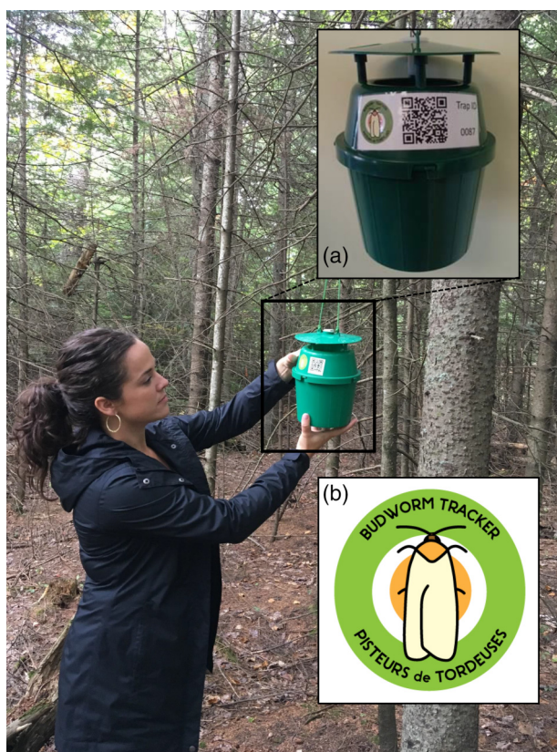
Fig. 2. A volunteer checking one of the Budworm Tracker traps that has been suspended from a lower crown branch of a host tree. (a) A close-up view of the trap and the label with its unique QR code, a Trap ID number, and (b) the Budworm Tracker logo (bilingual English/French).
